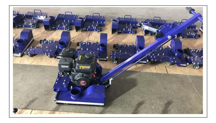
The Sidewinder crack chaser was designed to cut to depths up to  $\frac{1}{2}$ ".
